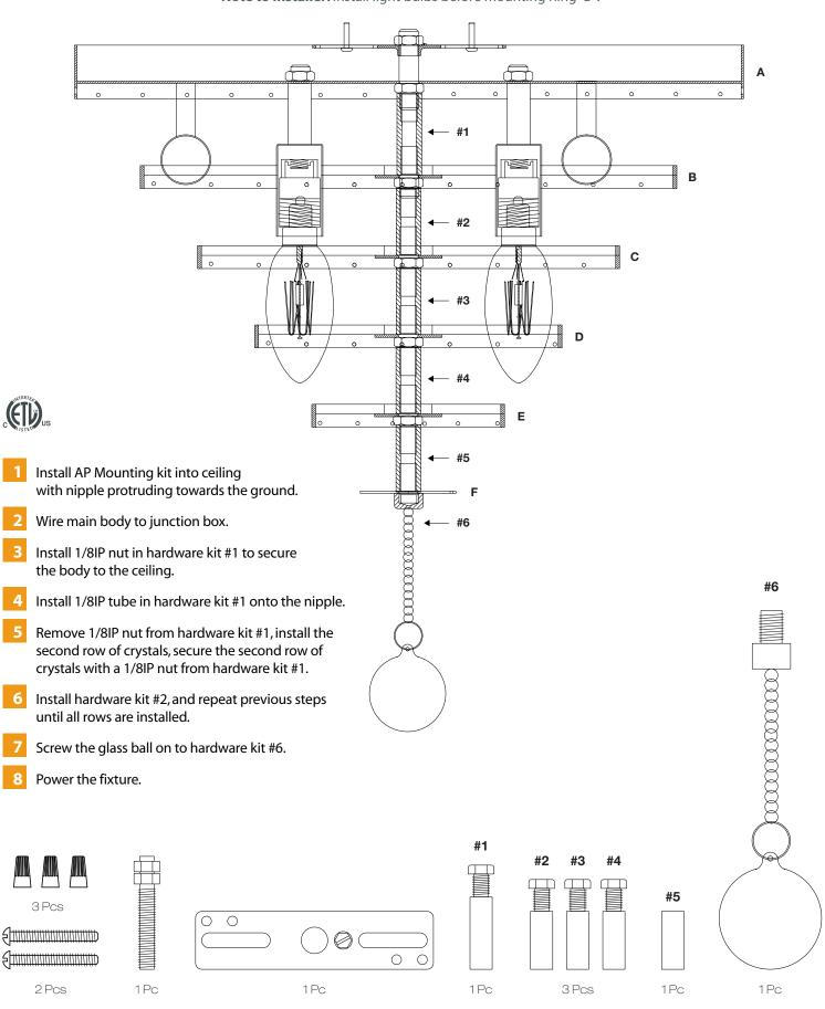
Note to Installer: Install light bulbs before mounting Ring "B".
